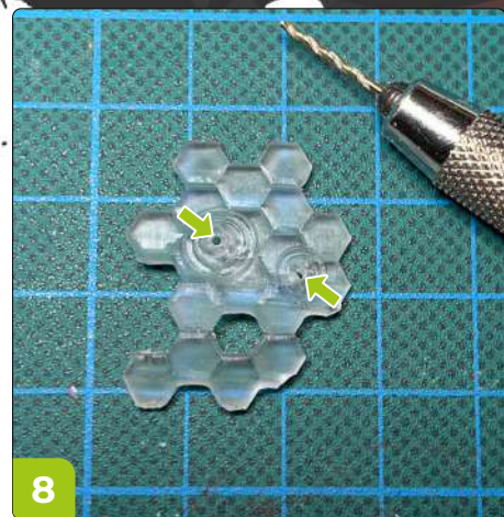
8. Remove the Shield Effect from the sprue, clean up any sprue stubs, and drill holes through the centre of the 'impact' effects.
