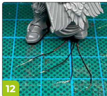
12. You will now need to trim the wires emerging from the feet so you have approximately 2cm of each wire still exposed, as shown in the image. Remember to keep the marks showing which are the two positive wires.
